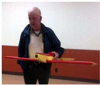
Leroy Brooks shared his electric converted 40 sized Super Sportster. He took the plans and reduced all wood down by one size from the recommended size. This made the plane very light; it weighs about a 1/3 of what the regular model weighs. It is covered by Monokote.
