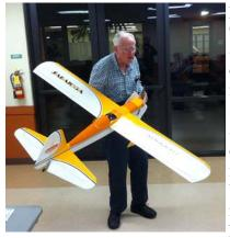
pictures of Charlie's plane and scaled it up to construct a new fuselage from scratch. He used an 80 amp speed controller, a 46 motor and a lipo battery. He will fly it the next time he is out at the
