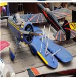
Mitch bargained for, but he's plugging along like a true builder. So far he's removed the wing-mounted retracts and is going with a hand-made carbon fiber fuselage-mounted main gear (fixed). He wasn't happy with the yard-stick (no kidding) main spar and really non-standard wing construction. We were both really perplexed as to why there was fabric covering on the underside of the wing skins. Mitch is also re-
