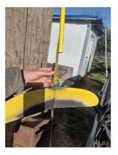
This is Steve's Micro RC glider kit by J&h Aerospace that uses a rocket pod to carry it to 800 feet before separating for the return home. It can also can be used as a discus hand launch guider
