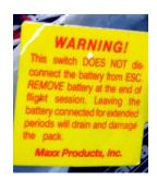
For larger models, a shorting plug should be used to totally isolate the battery from the ESC:
